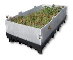
SOPRANATURE's TOUNDRA BOX is a pre-vegetated modular tray system. It is composed of a box made of 100% recycled polypropylene and removable, recyclable white belts, containing a filter fabric and a growing medium in which a mix of sedum species is cultivated. The mix of sedums can be adapted according to the hardiness zone and climatic conditions. The TOUNDRA BOX system can be installed on SOPRANATURE green roofs, garden terraces, and
